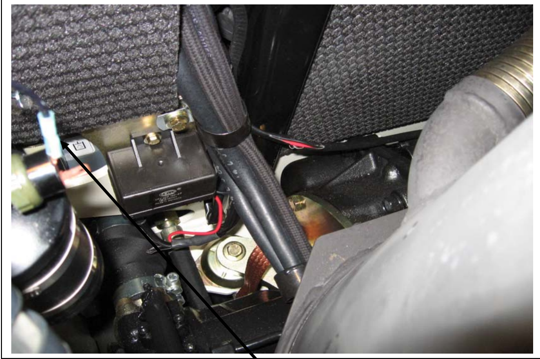
White 14ga clutch wire from evaporator.
