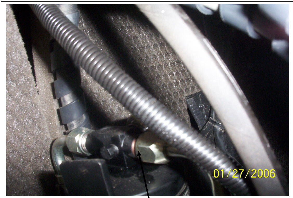
Hoses going through previously drilled holes in the panel into engine compartment
