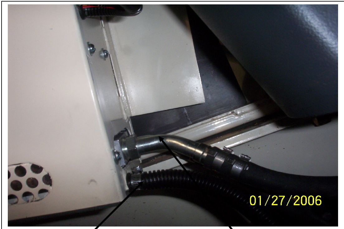
Drain tube connected.
