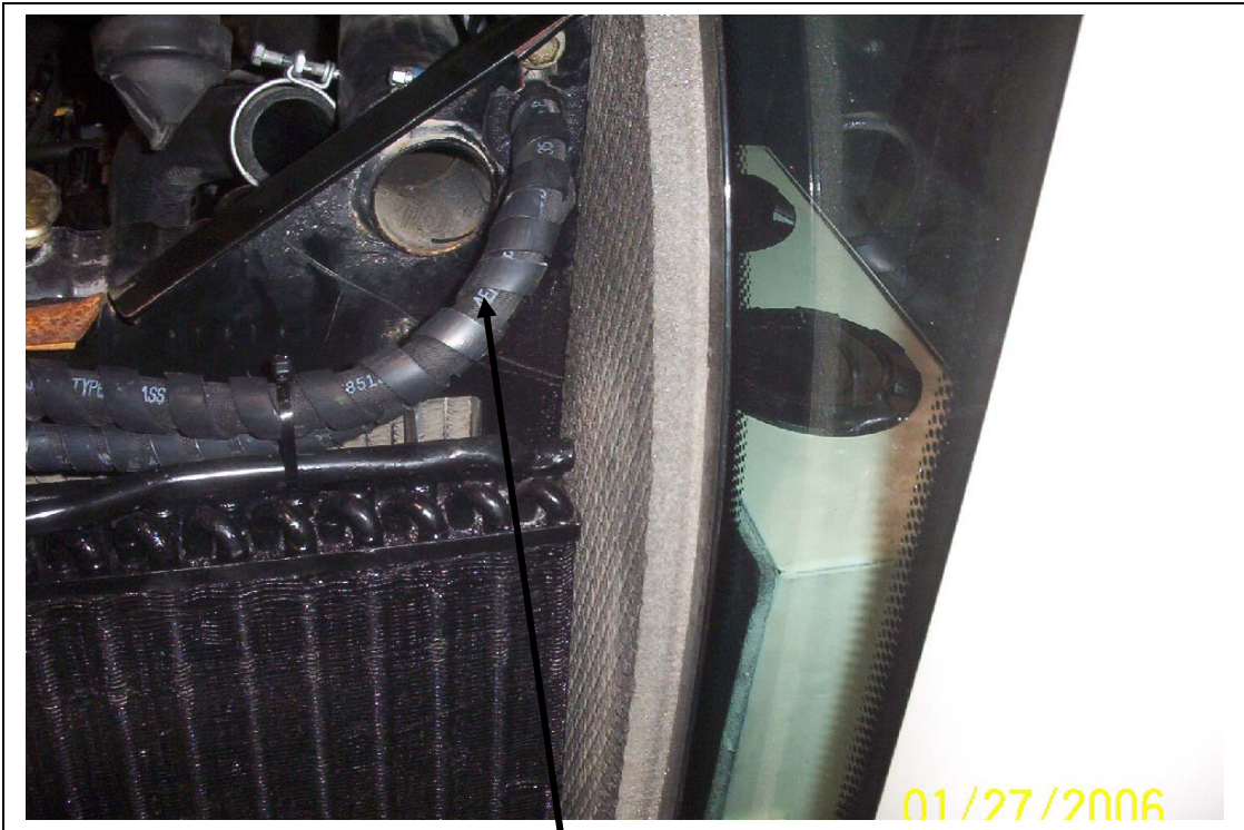
Hoses going through previously drilled holes in the panel into engine compartment
